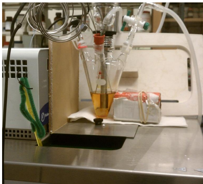
Figure A.2 Nanoparticle reactor equipped with a sonicator probe to mix magnetic nanoparticles.
