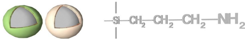
Figure I.1 Fe 3 O 4 /NH 2 substrate for Surface modification of MNPs
