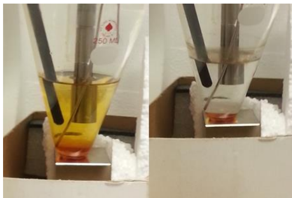
Figure A.3 Nanoparticle wash with anhydrous ethanol.
